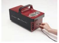
Connect the Control Unit to the AC Adapter, then to a grounded electrical outlet.
